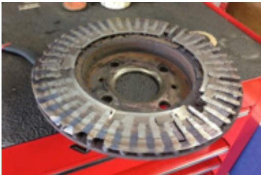
This rotor is also worn into cooling fin area
