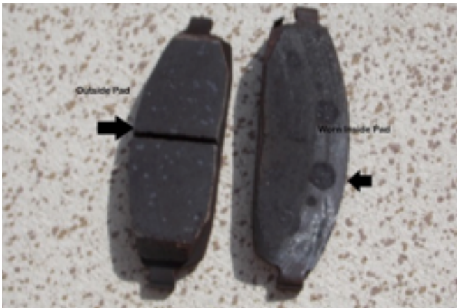
Brake pads showing extreme wear on one pad
