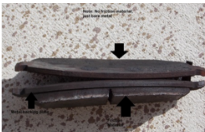
One brake pad with no friction material and one good pad
