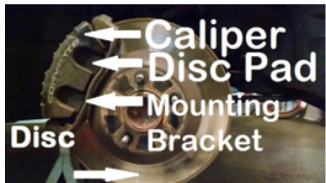
Disc brake components (at wheel)
