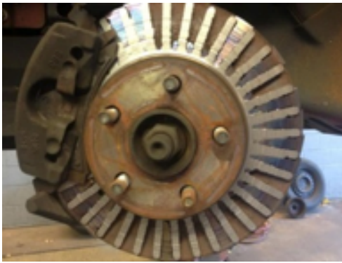
Rotor disc worn into cooling fin area
